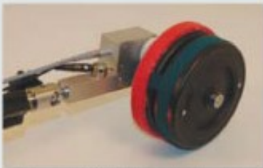
Wheel electrode with moistening wheel for continuous wetting up to a length of 200 m (650 ft). Linear distance recorder with travel direction detection. Automatic measurement of pre-selected intervals.
