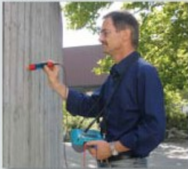
Measuring with rod electrode according to standards.
