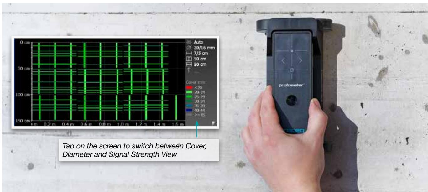
*Tap on the screen to switch between Cover, Diameter and Signal Strength View*
